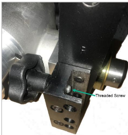
Rail Drill Rail Shoe Location
