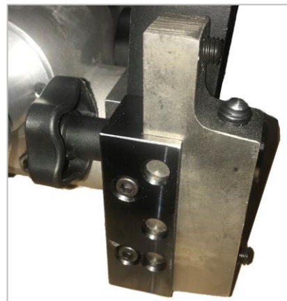
Properly Installed Rail Shoe
